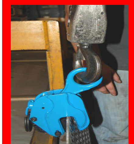
Bale leans to the left; hoist hook supports the bale.
