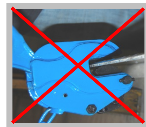
Improper Horizontal Lift
